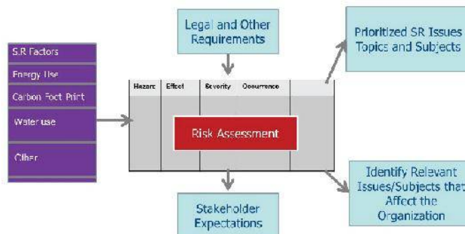
FIG.3 . Integrated risk assessment methodology for EMS including Energy, Social Responsibility (SR) and Sustainability . [7]
